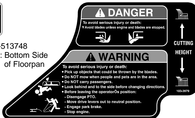
PART NO. 103-3979 LOCATION: RH Side of Console
