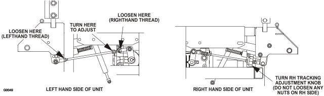
NOTE: The nut to the front of the unit on the LH rod has left-hand threads. FIGURE 18
