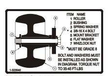
PART NO. 1-323540 LOCATION: Left Rear Corner Top of Mower Deck
