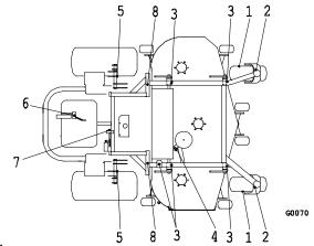
c) Lubricate front caster pivots once a year. Remove hex plug and cap.
