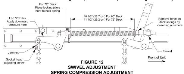
Raise deck lift lever to the 5" (12.7 cm) cutting height position See Figure 10. Adjust spring compression until proper distance is obtained between the two large washers (See Figure 12). Adjustment is made by turning the nut at the front of each spring (clockwise will shorten the spring, counter-clockwise will lengthen the spring). Lock in position with jam nuts.
