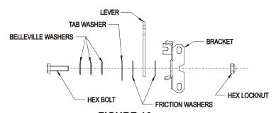
FIGURE 16 THROTTLE TENSION
