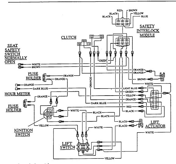
Console Wiring Diagram
