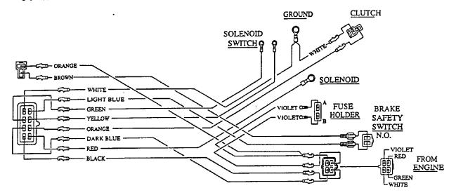
Engine Deck Wiring Diagram
