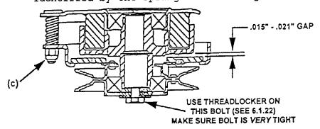
FIG. 12 ELECTRIC CLUTCH ADJUSTMENT
