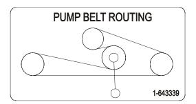
PART NO. 1-643339 LOCATION: Top of Right Engine Baffle
