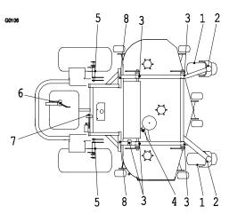
c) Lubricate front caster pivots once a year. Remove hex plug and cap. Thread grease zerk in hole and pump with grease until it oozes out around top bearing. Remove grease zerk and thread plug back in. Place cap back on.
