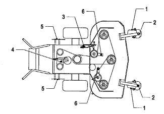
c) Lubricate pivot points with a spray penetrating lubricant as directed below.
