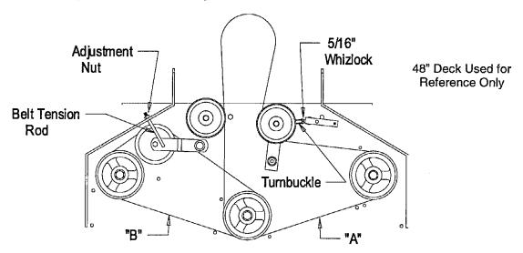
FIG. 11 CUTTER DECK BELT ADJUSTMENT
