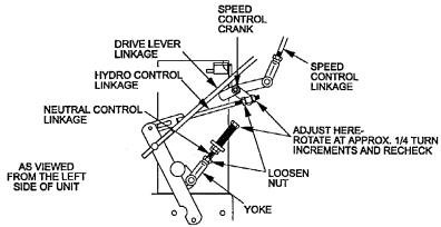
FIG. 14 HYDRO DRIVE LINKAGE ADJUSTMENT
