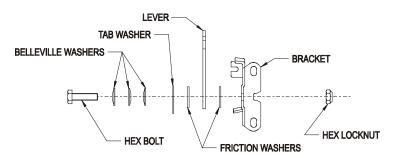
FIG. 12 THROTTLE TENSION
